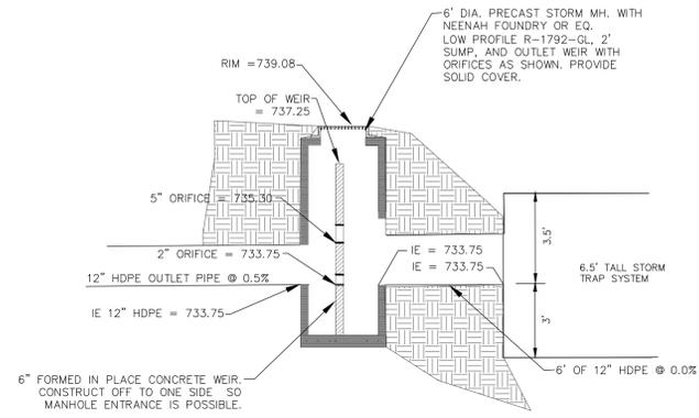
**OUTLET STRUCTURE B DETAIL**
